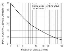
FIG.5 MAXIMUM NON-REPETITIVE FORWARD SURGE CURRENT
